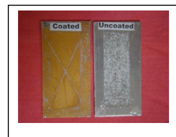
Photographs of coated and bare AA2024-T4 substrates after 168 hrs of salt spray test
